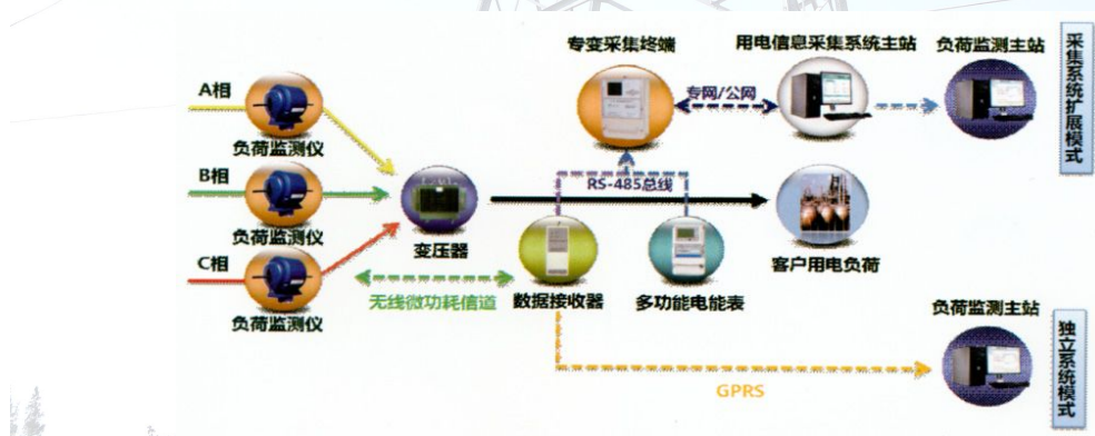
2 - 1 Topology of the anti-theft monitoring system
